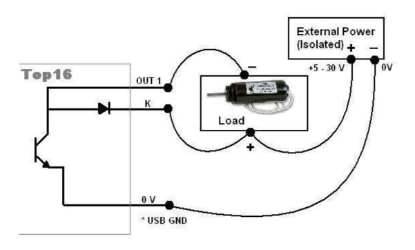
Each output is the collector of a transistor which effectively connects the output to 0V (when output is ON) and will sink up to 250mA (all outputs on) or 350mA (single output on). When the output is OFF it is a high impedance.
